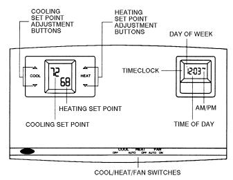
Fig. 3 — TEMP System Thermostat (With Timeclock Shown)
